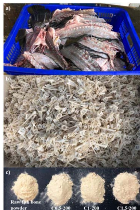
Figure 1. a) Lates calcarifer seabass bone; b) white bones after removing all organic matters; c) Raw fish bone powder and calcium powder samples obtained by alkaline hydrolysis at 200°C for different times (0.5; 1; 1.5 hours).
